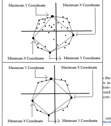
Fig. 4. Elimination of points within triangle.
